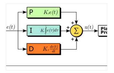
rightServo.writeMicroseconds(1500 + iniMotorPower - Kp\*error); leftServo.writeMicroseconds(1500 - iniMotorPower - Kp\*error);
