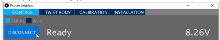
**! The battery voltage should be around 8.0–8.4V.**
