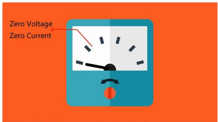
Étape 3 - The multimeter must be placed horizontally when used to avoid errors.
