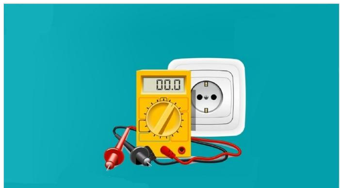
Étape 4 - Do not touch the metal part of the test lead with your hands to ensure accurate measurement and personal safety.
