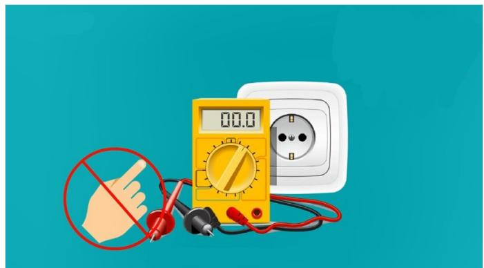
Étape 5 - When measuring a certain amount of electricity, especially for high voltage or large current, you cannot shift gears while measuring, otherwise the multimeter will be damaged.
