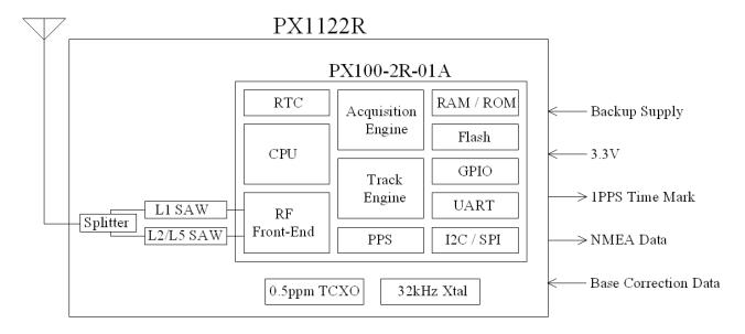
Active antenna is required to use with PX1122R. The received signal goes through a signal splitter, to individual L1 and L2/L5 SAW filters to remove out-band interference, then to the PX100 GNSS receiver chip for RTK signal processing. Using correction data from an RTK base station, the rover PX1122R computes its position to centimeter-level accuracy relative to the base station.
