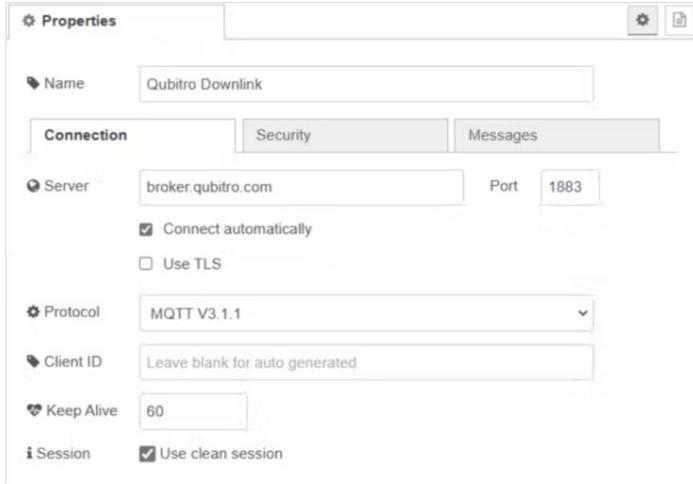
The screenshot shows the 'Properties' window for an MQTT Out node in Node-Red. The 'Name' field is 'Qubitro Downlink'. The 'Connection' tab is selected. The 'Server' is 'broker.qubitro.com' and the 'Port' is '1883'. There are checkboxes for 'Connect automatically' (checked) and 'Use TLS' (unchecked). The 'Protocol' is set to 'MQTT V3.1.1'. The 'Client ID' is 'Leave blank for auto generated'. The 'Keep Alive' is '60'. The 'Session' checkbox 'Use clean session' is checked.
