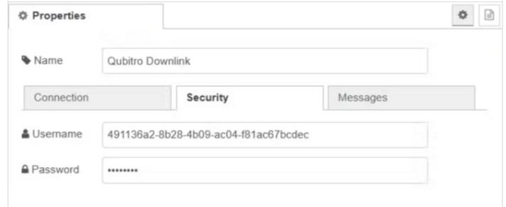
The screenshot shows the 'Properties' window for an MQTT Out node in Node-Red. The 'Name' field is 'Qubitro Downlink'. The 'Security' tab is selected. The 'Username' is '491136a2-8b28-4b09-ac04-f81ac67bcdec' and the 'Password' is masked with '\*\*\*\*\*'.
