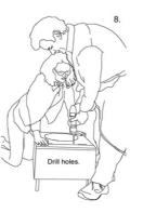
When screwing the legs to the inside of the box, make sure the top edge of the box will sit about 1/2" below the top edge of the receptacle (the top of the rim should protrude through the box by 1/2"). This allows the rim to sit tight against the underside of the toilet seat (which is why the toilet seat bumpers are pried loose and swiveled to one side, as shown in #5 and #6).
