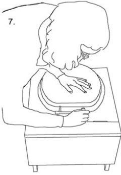
7. Mark holes for toilet seat attachment.
