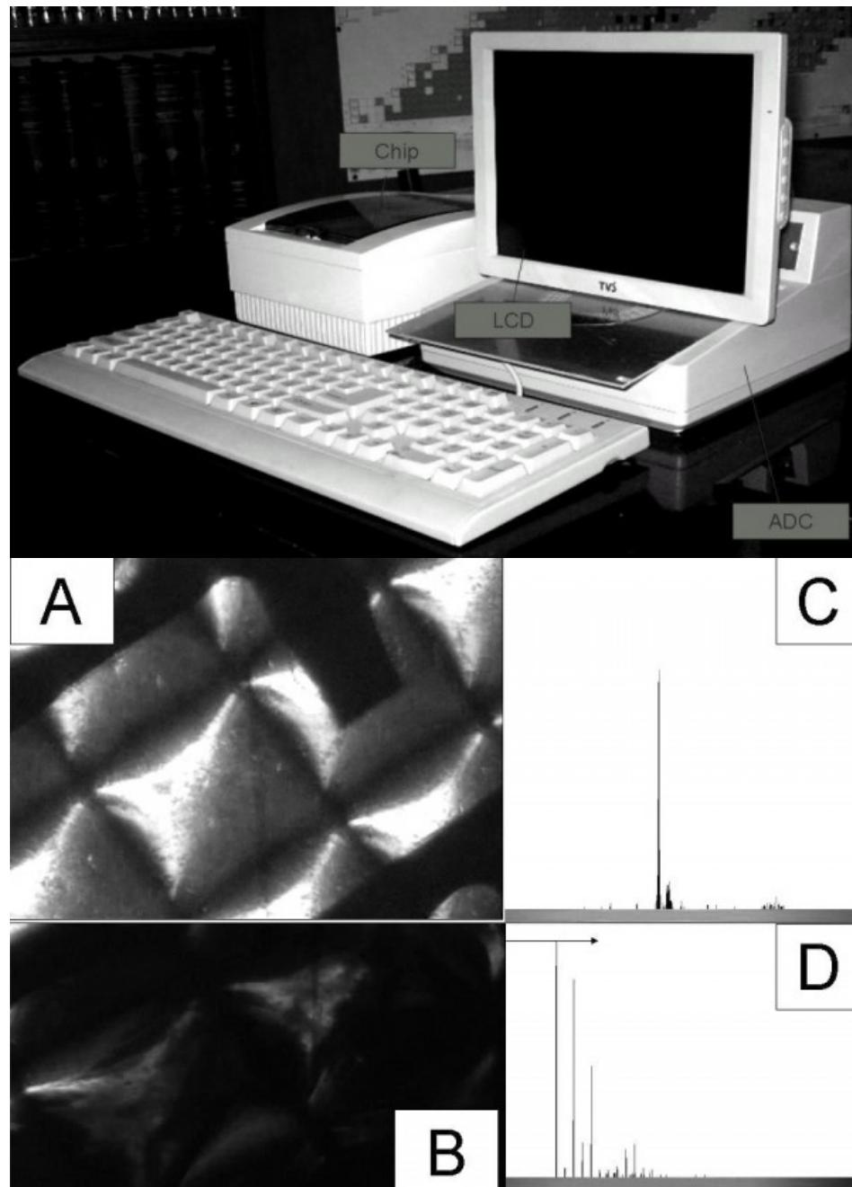
Redox-signal conversion into the optical signal using colorimetric / spectrophotometric “chemical pixels” (“chemical resells” / “sensels”): A,C – baseline (reactive film without detective dye response); B,D – indicator signal. Equivalent mosaic sensor-converter elements may be assembled using different converters and indicators (not only “pH-pixels” / “pX-pixels”, but also “electric luminescence pixels”, “magnetic field pixels”, “radiation pixels”).
