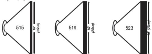
Different fan width - same orifice sizes: The example below demonstrates the difference between tips with the same orifice size, but increasing fan sizes. The same amount of coatings is applied over a larger area - or less coating per square inch using the same pressure and hand-speed as you spray. When necessary, remember to size up or down your orifice as you size up or down your fan width if you want to apply the same amount of coating per square inch.
